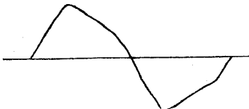
Fig. 6. Waveform of output voltage for an approximately sine wave input.
